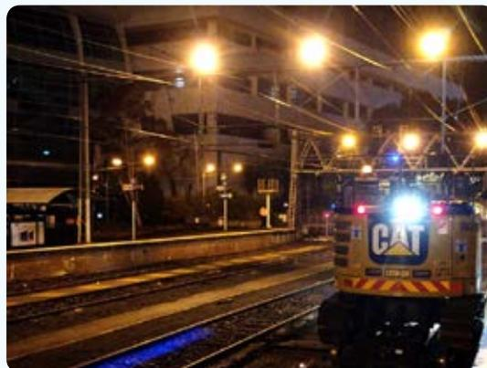
spot or in close proximity. If the system detects a person or plant in the vicinity, the halo system and dashboard lights start flashing to create an alert for the driver and nearby workers.”
