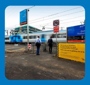
Metro has also managed upgrades funded by the Department of Transport to reduce risks at level crossings. Electromagnetic escape gate latches on existing crossings have been installed. Improvements to the design height of existing crossing locations with electromagnetically latched escape gates at a number of high priority sites prevent pedestrians accessing the tracks while the crossing is closed.
